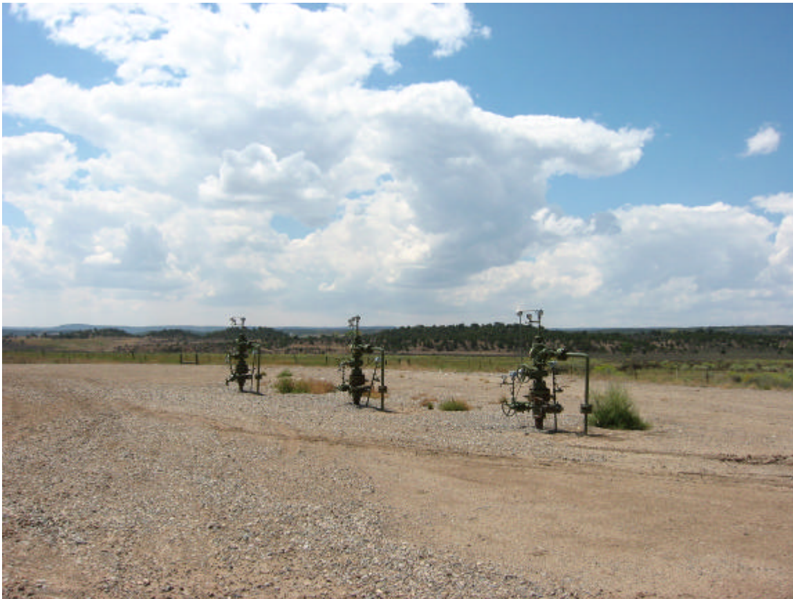
Figure 16: Proximity of Injector Wellheads to One Another, Tiffany Unit
